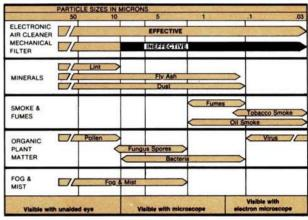
Chart used to dramatize the comparative size of various pollutants and the superior efficiency of the Precipitator on particles not visible with the naked eye.
